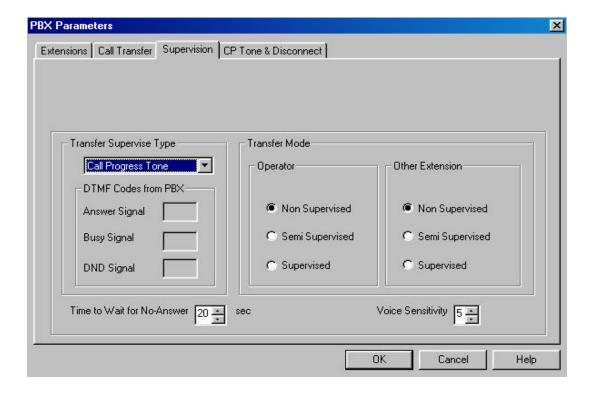
**Transfer Mode** – This is where the operation mode is selected for the Voice Mail's Auto Attendant. **Non-Supervised** is when the Voice Mail transfers the call without checking the status of the extension, **Semi-Supervised** is when the Voice Mail only recognizes the busy signal from the PBX and **Supervised** is when the Voice Mail check for busy signal from the PBX and no-answer time out. Command: \*350
