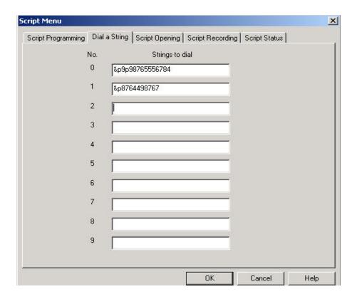
This is the table for the DTMF strings to dial. A string can be up to 20 digit including A-D, 0-9,\*,#, p for pause and & for Hook Flash.
