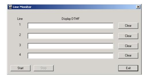
The line monitor is a powerful tool used to make integration easier. The Line Monitor shows all incoming DTMF signals, on-line, simultaneously, from all four ports via the RS 232 cable.
