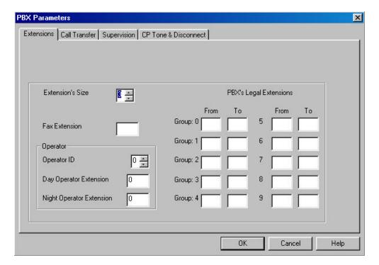
**Extension Size** – The PBX extension size needs to be defined. This refers to the numbering plan of the PBX, for example: if the extensions in the PBX are from 200 to 299, then the extension size is 3 digits. Please note that 2, 3 or 4 can be used and the default is 3.
