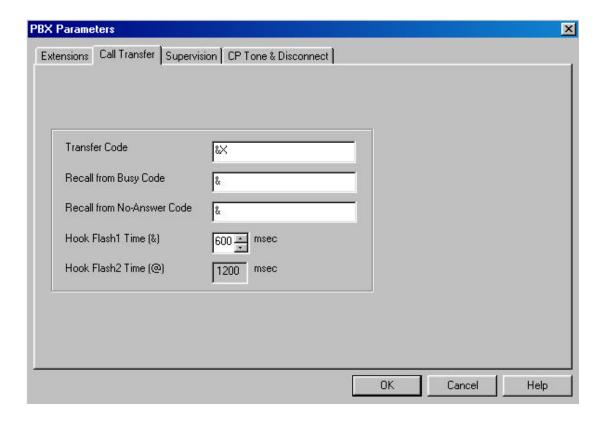
**Transfer Code** - This code is used to transfer a call from an analog extension to another.
