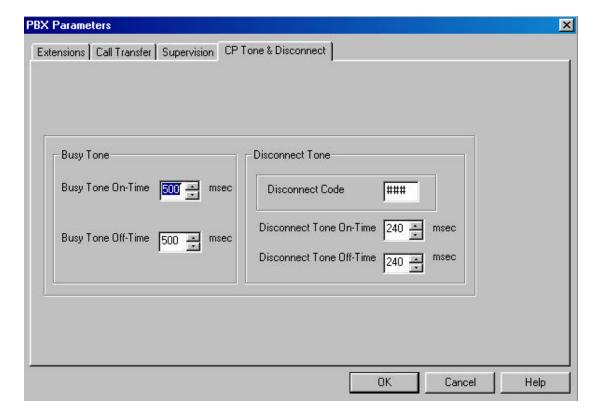
**Busy Tone** – The "Busy on-time" and the "Busy off-time" determine the busy tone cadence. Busy tone is used for: a.) detecting a busy extension when transferring a call in semi or supervised transfer mode and b.) disconnecting the line when detecting a disconnect situation.
